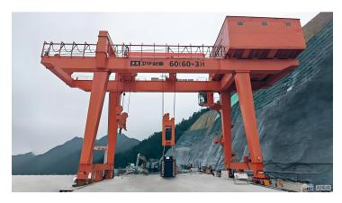
The 60 tons gantry crane is a professional heavy-duty material handling solution engineered to meet the rigorous demands of high-capacity lifting in industrial, port, and construction environments. Designed for reliability, efficiency, and safety, this crane delivers consistent performance when moving loads up to 60 metric tons, making it a cornerstone asset for businesses requiring robust lifting capabilities.
