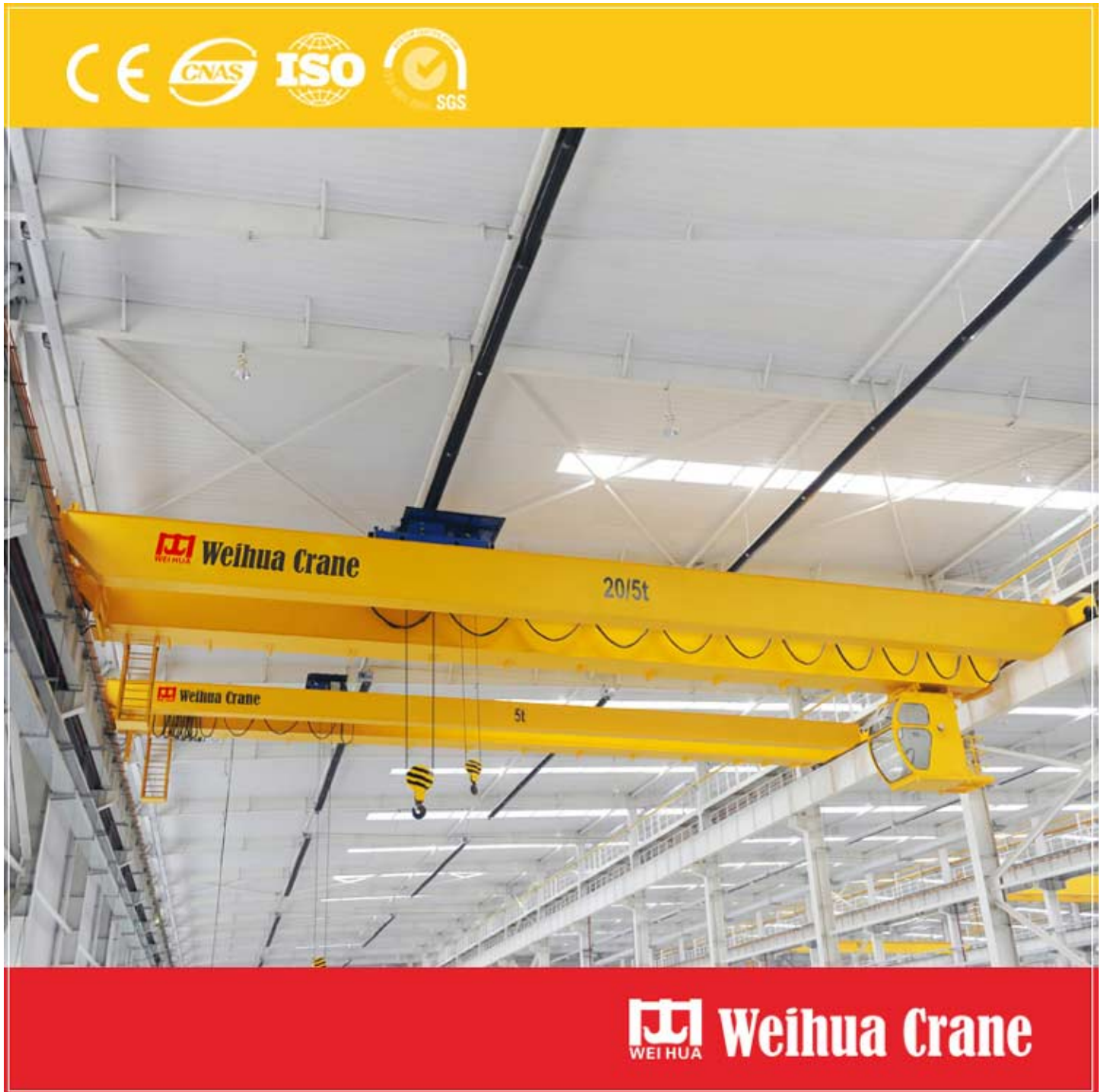
double girder overhead crane
