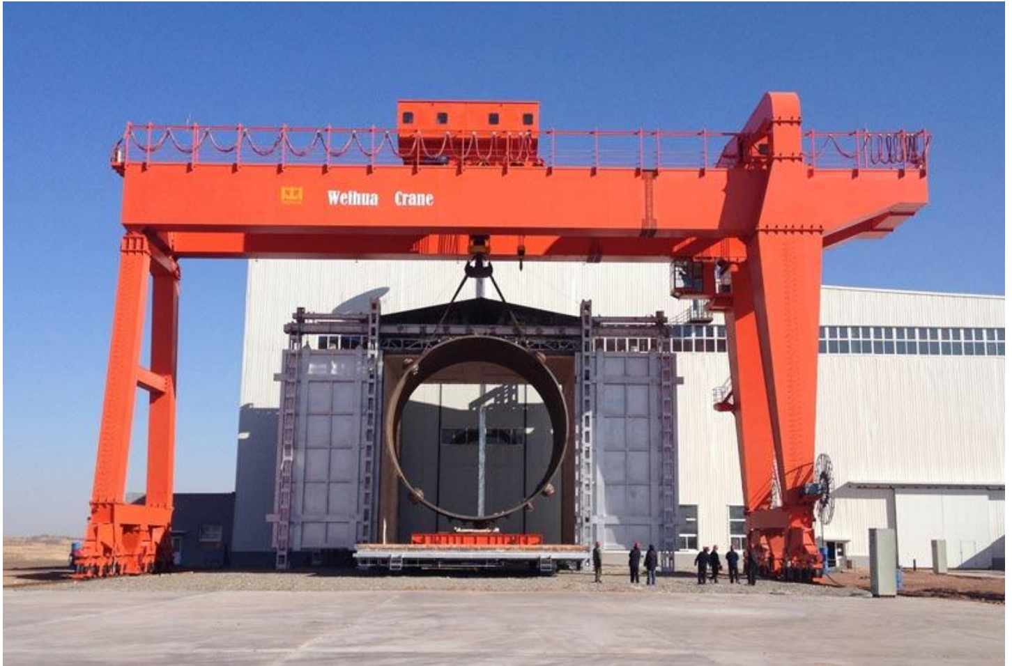
Mobile Double Girder Gantry Crane
