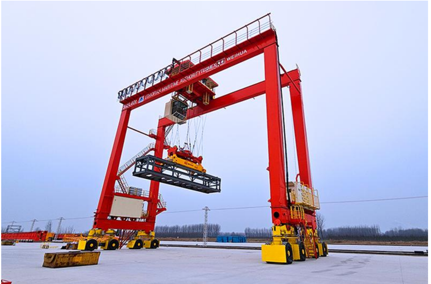
RMG Container Gantry Crane (Rail-Mounted Gantry)
