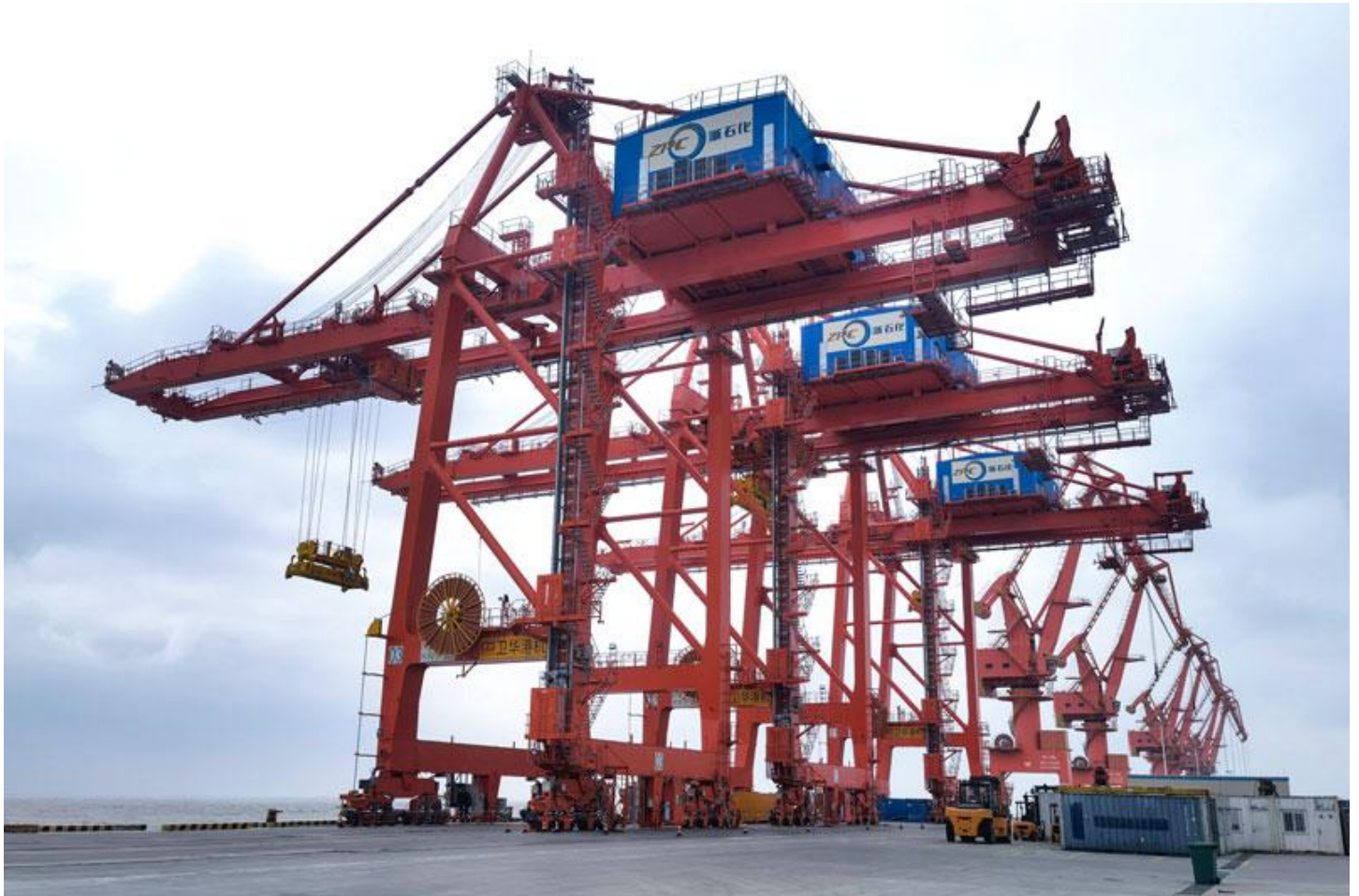
STS Container Gantry Crane (Ship-to-Shore)
