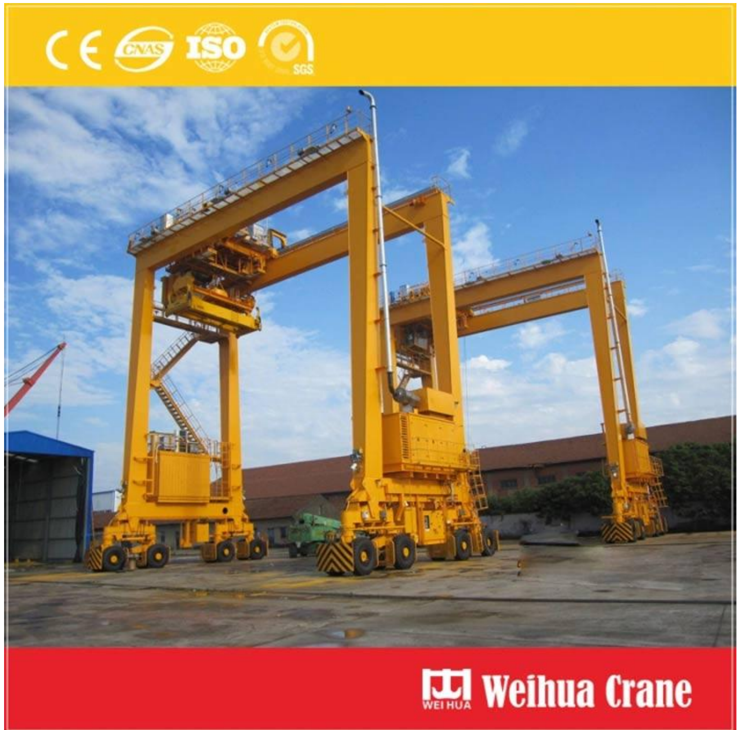
50-ton RTG container crane used in ports
